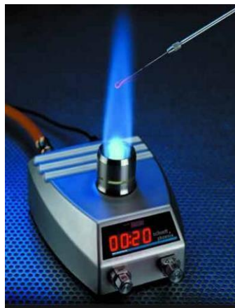
(B) Automatic gas burner
